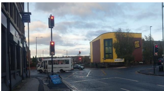
Queens Road approach to junction. Banned right turn signs on double signal head
